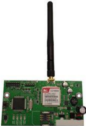
FIGURE 11 - SMS ALARM MODULE
